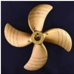
Figure 4 Photo of the model propeller.
