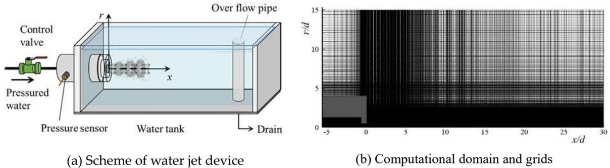
Figure 1. Scheme of submerged water jet and computation domain of numerical simulation.
