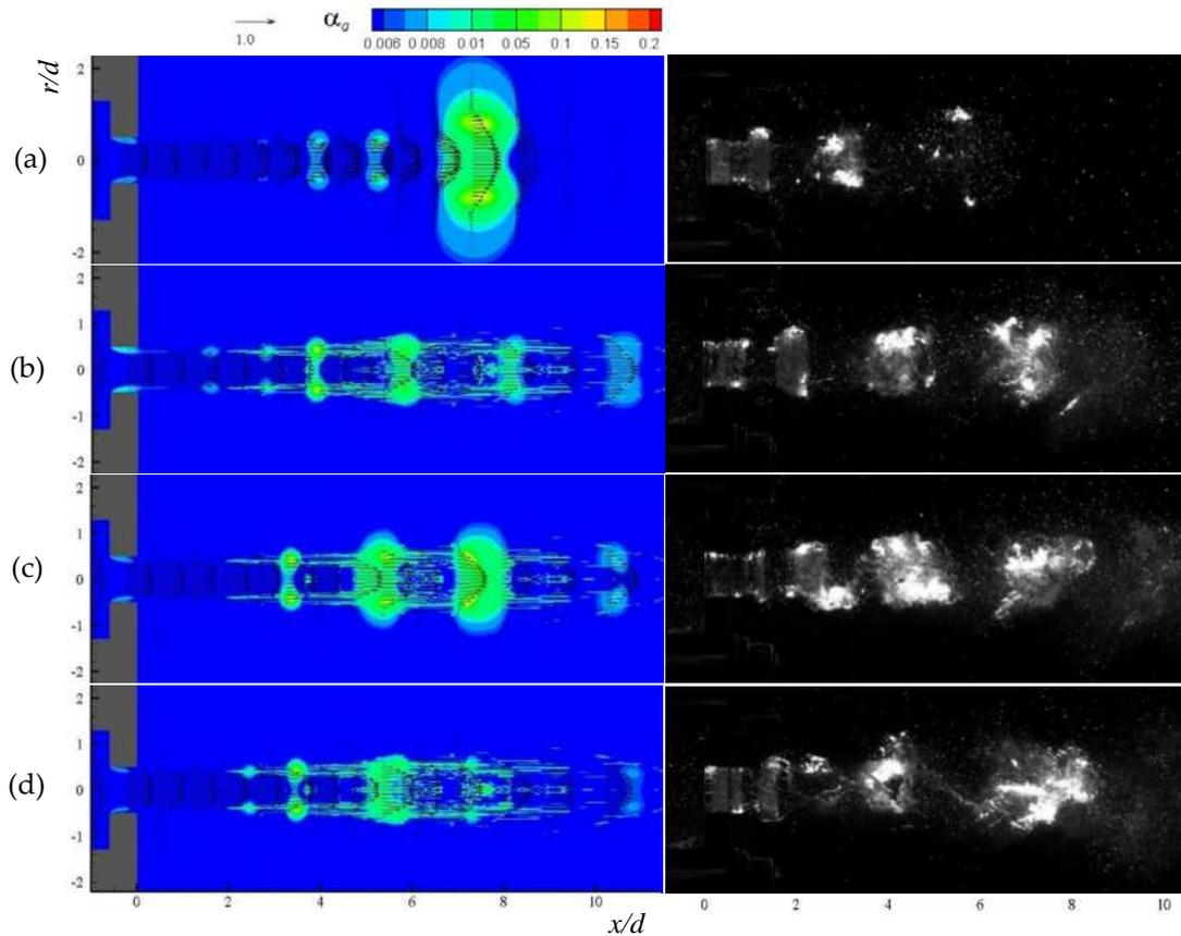
Figure 2. Distribution of cavitation clouds in submerged water jet obtained by numerical simulation (left) and high-speed video camera observation (right): (a)  $t = t_1$ , (b)  $t = t_1 + \Delta t_1$ , (c)  $t = t_1 + \Delta t_2$ , (d)  $t = t_1 + \Delta t_3$ .
