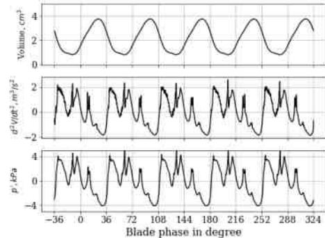
Figure 2 Vapor volume and hull pressure pulse in blade phase series. Top frame: integrated total vapor volume; middle frame: second order derivative of total vapor volume; bottom frame: pressure history at transducer No. 7.
