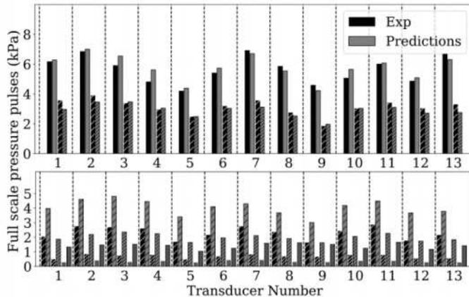
Figure 1 Predicted hull pressure pulses and comparison with experimental measurements. Upper frame: 1st and 2nd BPF; lower frame: 3rd to 5th BPF. Values are reported in full scale.
