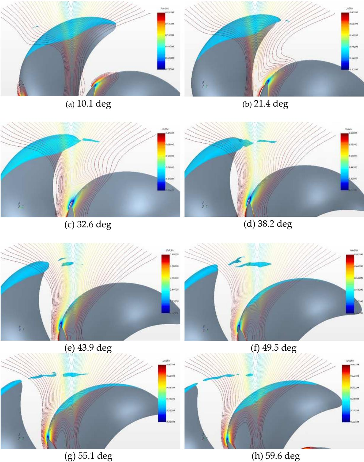
**Figure 1.** Cavitation (iso-surface of  $\alpha_v = 0.5$ ) history with axial propeller inflow slightly upstream the propeller blade.
