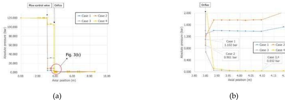
Figure 3. Variation of absolute pressure according to the location: (a) The whole analysis model; (b) Nearby orifice.
