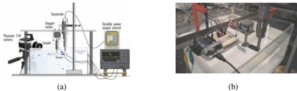
**Figure 1.** a) Sketch of the experimental setup showing the liquid container, instrumentation and equipment; and b) Photograph of the emerging platform of ultrasonic cavitation system.
