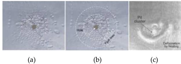
**Figure 3.** Cavitation erosion on aluminum. Image (a) and (b) are, respectively, original and digitally-processed images of the 6  $\mu\text{m}$  aluminum foil eroded during 10 s at 50%; (c) 50  $\mu\text{m}$  aluminum foil irradiated by 60 s.
