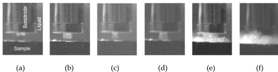
**Figure 5 (a-f).** Cavitation on a clean surface. Formation of a vaporous layer on both surfaces, on the upper surface the vaporous flow is centered, with  $\phi = 4$  mm and on the lower surface it is expanded reaching 30 mm in diameter. File: Test 9-100%, 34000 fps, 640x480 resolution.
