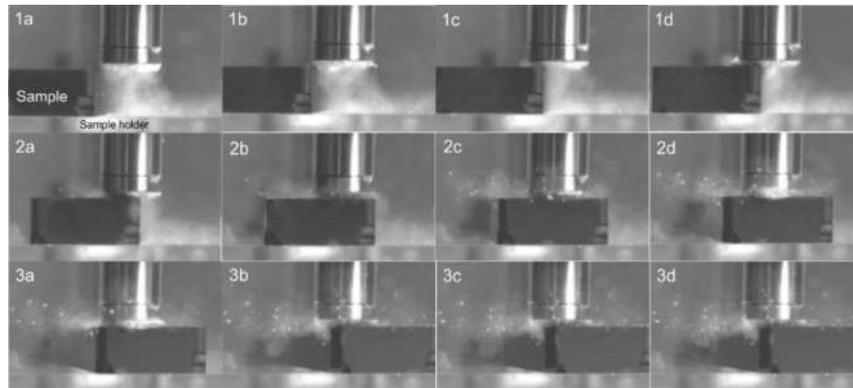
**Figure 6.** The sample rotates at 48 Hz, the intensity is set at 100%,  $h = 1.16 \pm 0.14$  mm, the tip is submerged 23.5 mm. (1a) - (1d) Pulsating cavitation cloud begins its sweep over the sample surface; (2a) - (2d), expansion and compression of the confined cloud; and (3a) - (3d) ejection of fluidic structures at a speed of  $2\text{ms}^{-1}$  at the exit of the sample surface. Resolution 256x256.
