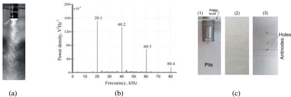
**Figure 2.** a) Acoustic field generated by the transducer at 100% power and immersed 23 mm in water. A cloud attached to the sonotrode tip and an inhomogeneous axisymmetric field can be observed; b) Power density vs. frequency at 70%, showing fundamental, harmonic and subharmonic peaks; c) Images of the aluminum foils before and after exposure to ultrasonic cavitation, showing antinodes and pits on its surface.
