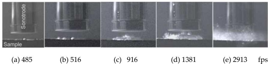
**Figure 4.** Ultrasonic cavitation process generated on a simple hard surface. Ultrasonic irradiation at 100% on unpolished ceramic Y 35 for 285 ms. Fast video is acquired at 49000 fps with resolution of 512x384.
