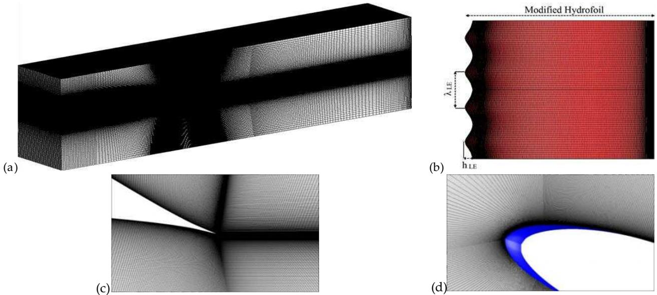
Figure 2. 3D structure grid generated around the NACA 634-021 hydrofoil.
