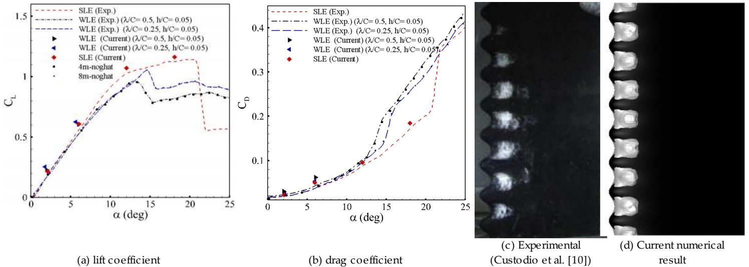
Figure 3. Comparison of the (a, b) force coefficient and (c, d) vapor volume fraction with the experimental data
