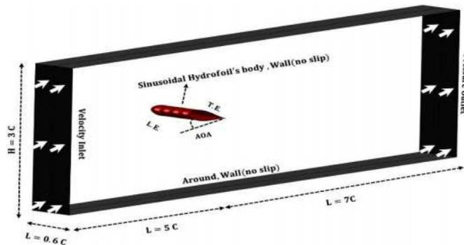
Figure 1. 3D view of the computational domain with boundary conditions.
