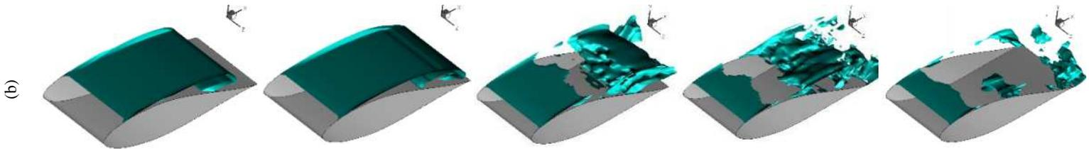
Figure 4. Iso-surfaces of volume fraction ( $\alpha=0.5$ ) in one complete cavitation cycles ( $\sigma=0.8$ ) for (a) WLE and (b) SLE hydrofoil.
