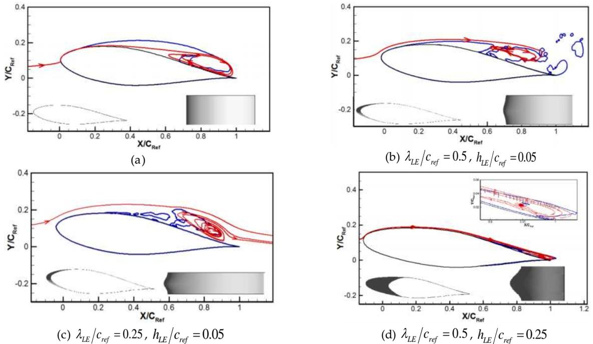
Figure 6. The visualization of the re-entrant jet pattern (displayed with streamlines mean-velocity) (red lines) and time-averaged volume fraction (blue lines) ( $\sigma=0.8$ ).
