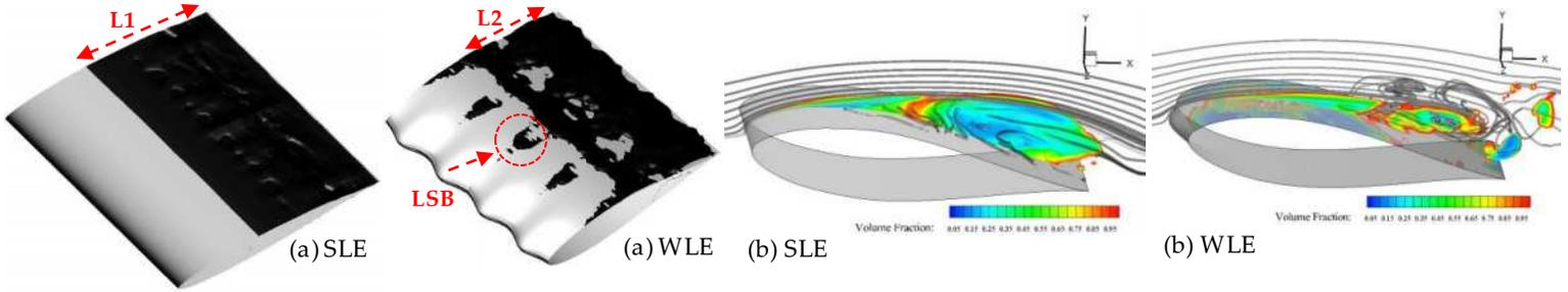
Figure 5. The comparison of the isosurface of zero velocity (a), and the volume fraction with streamline (b) over the WLE and SLE hydrofoil ( $\sigma=0.8$ ).
