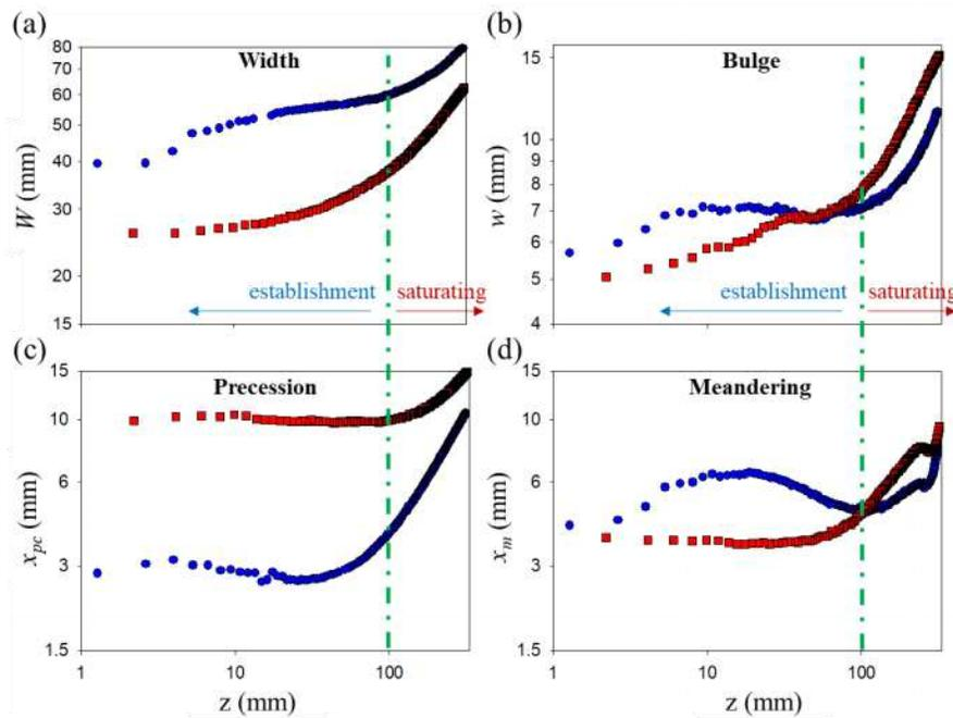
Figure 2. Bubble plume kinematics parameters (a) time averaged width, (b) bulge, (c) precession and (d) meandering for ●: conventional bubble plume, ■: churn-turbulent bubble plume
