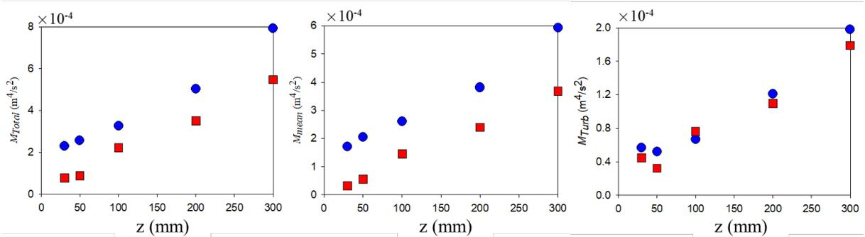
Figure 3. Time averaged integrated (a) total momentum flow rate, (b) mean momentum flow rate, (c) turbulence momentum flow rate for ●: conventional bubble plume, ■: churn-turbulent bubble plume
