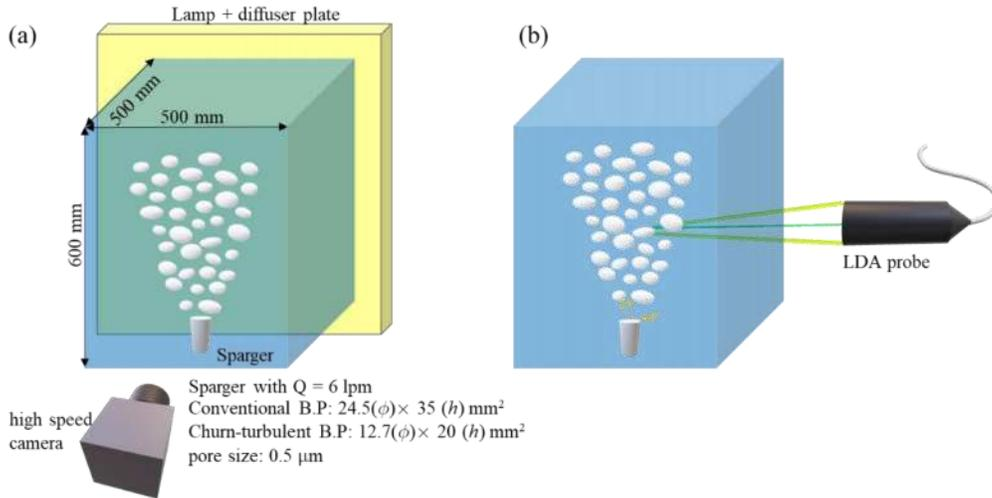
Figure 1. Experimental setup for (a) gas phase measurement (shadowgraph technique) and (b) liquid phase measurement (laser doppler anemometry)
