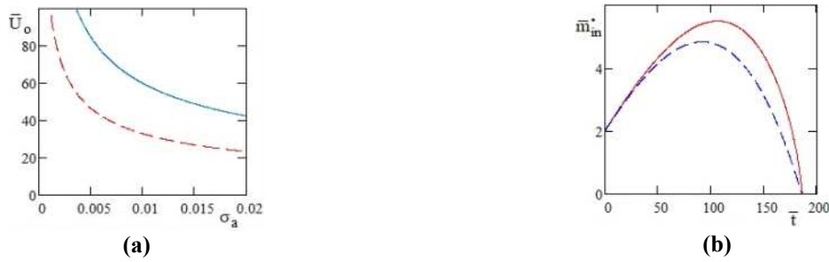
Figures 5. a) Limitations of the range of velocities at the initial moment \bar{U}_0 = \bar{U}_0(\sigma) , corresponding to the proximity of the forms of non-stationary and stationary cavities: ——— eq. (11b), - - - - almost complete coincidence, in the maximum radius accurate to 0.9R_k ; b) Intensity of mass gas injection Eq. (12-13) providing the proximity of non-stationary and stationary caverns at uniformly accelerated motion at \sigma_a = 0.02 , \kappa_c = 0.5 , \bar{P}_\infty = 500 , t_{co}^0 = 15^\circ , \bar{t}_0 = \bar{U}_0 = 36.5 : ——— calculation by adiabatic 1/n = \kappa = 1.4 , - - - - calculation by isotherm n = 1 .
