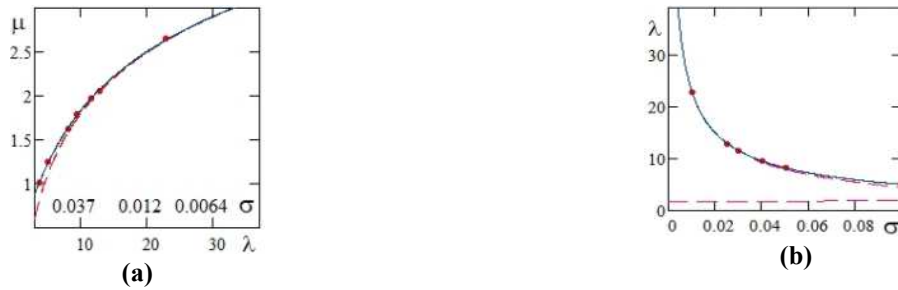
Figure 1. (a) Calculations \mu : ----- Eq. (3a) , ——— Eq. (3b), •••• nonlinear calculations [3]; (b) Calculations \lambda(\sigma) : ----- Eq. (3d), ——— Eq. (3c- 3e), •••• numerical calculations [3]
