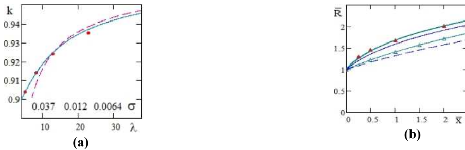
Figure 2. (a) Calculations k : ----- Eq. (4a), ——— Eq. (4b), •••• numerical calculations [3]; (b) The shape of the stationary cavity forward part: ——— experiments data [2], ▲▲▲▲ - numerical calculations for \sigma = 0.01 [3], Calculations : ——— Eq.(6b) for \sigma = 0.01 , ▲▲▲▲ Eq. (6a) \sigma = 0.04 , ----- Eq (6a), \sigma = 0.004 .
