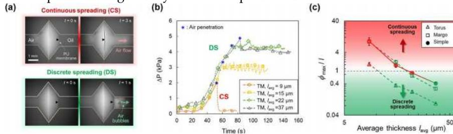
**Figure 3.** Consecutive air-spread through the TM-pit model. (a) Two types of air-spread: continuous spread (CS) and discrete spread (DS). (b) Temporal variations of  $\Delta P$  across the TM-pit models. (c) Two types of air spreading classified by the ratio of the maximum pore size  $\phi_{max}$  to the membrane thickness  $l$ .
