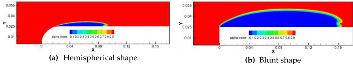
Figure 2. Cavity shape over the cylinder with different cavitator shape with  $Ca = 0.3$
