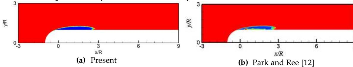
Figure 4. Velocity and streamline on a slice plane with cavitation number  $Ca = 0.3$
