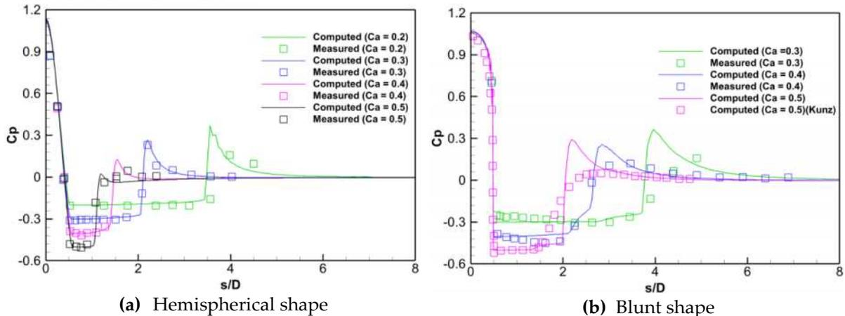
Figure 1. Comparisons of time-averaged surface pressure with different cavitation number
