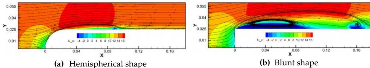
Figure 3. Velocity and streamline on a slice plane with cavitation number  $Ca = 0.3$
