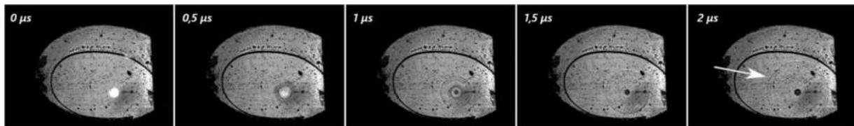
**Figure 1.** Cavitation bubble generates pressure waves, captured with high-speed camera.
