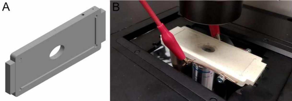
**Figure 2.** Custom made microscope chamber for generating single microbubble collapse with pressure waves. Schematic drawing of chamber (A) and experimental setup mounted on microscope table (B).
