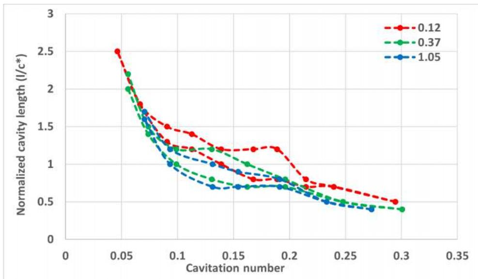
Figure 3. Normalized cavity length for three different non-dimensionalized thermal parameters.
