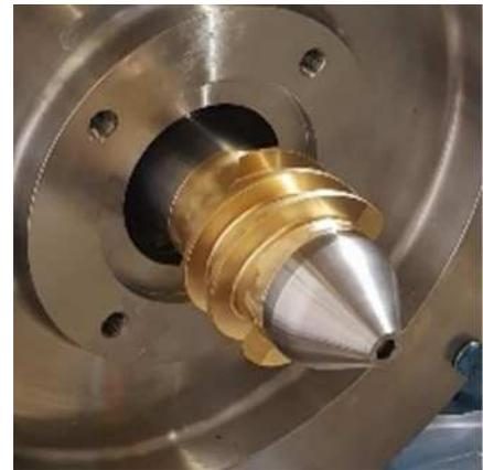
Figure 2. Two-bladed inducer.
