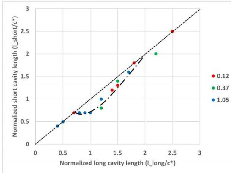
Figure 4. Cavity length difference between long cavity and short cavity.
