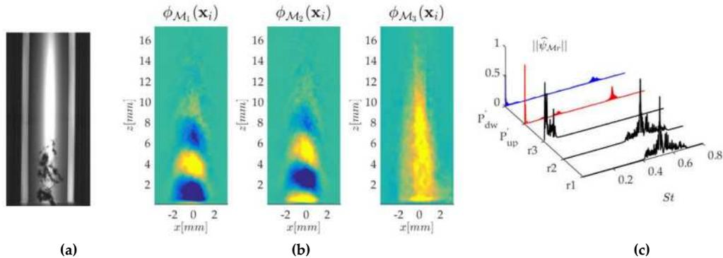
**Figure 4.** Cryogenic test case ( $\sigma = 0.89$ ): (a) Instantaneous image of the cavitating flow; (b) Spatial structures from the first three dominant mPOD modes; (c) Corresponding dimensionless spectra of the first three dominant mPOD modes together with the dimensionless spectra of the pressures upstream and downstream of the orifice.
