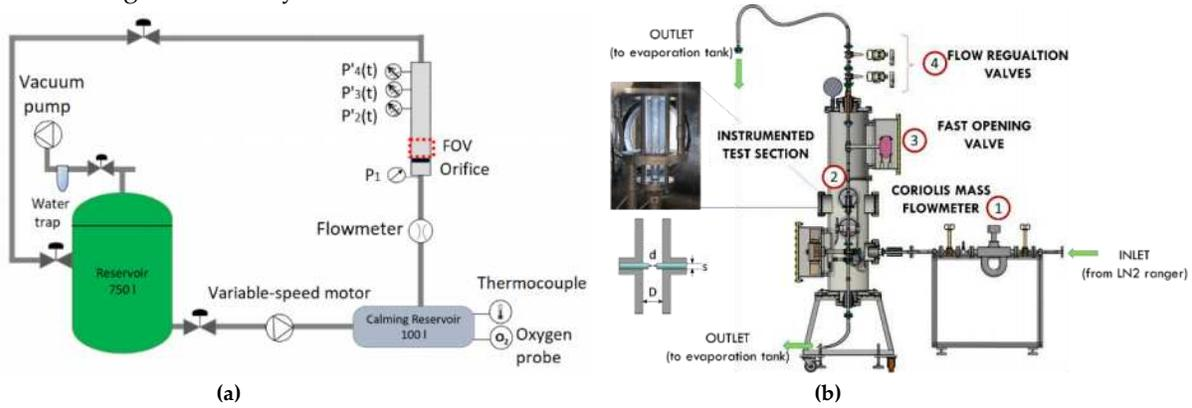
Figure 1 Schematic of the water closed-loop facility [9] (a) and the cryogenic facility [10] (b).
