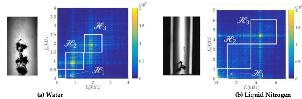
**Figure 2** Color plot of the spectrum of the correlation matrix: (a) Water at  $\sigma = 1.30$  with highlighted three scales  $\mathcal{H}$  [0–500, 500–1500, 1500–2500]; (b) Liquid Nitrogen at  $\sigma = 1.05$  with highlighted three scales  $\mathcal{H}$  ([0–1000, 1000–3500, 3500–6000]).
