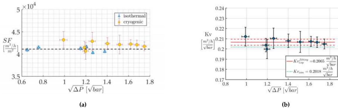
Figure 3. (a) Experimental SF calculated from the fitted  $Kv$ -water (dashed line) compared to the SF for each data point in fully liquid from the isothermal case (triangles) and from the cryogenic case (circles). (b) Comparison between the experimental and the theoretical  $Kv$  for the cryogenic case.
