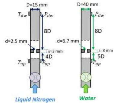
**Figure 1.** Sketch of the two test sections with their characteristic dimensions.
