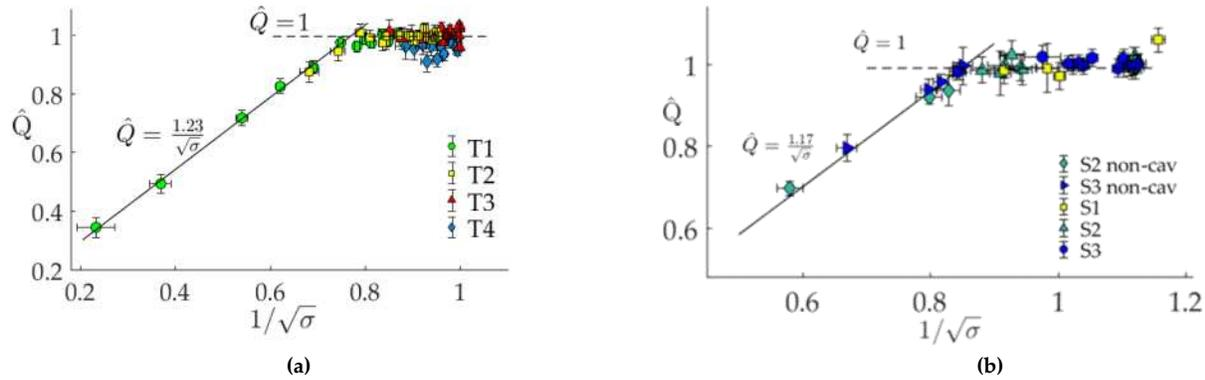
Figure 2. Dimensionless hydraulic curve for the two similar orifices with water (a) and LN<sub>2</sub> (b).
