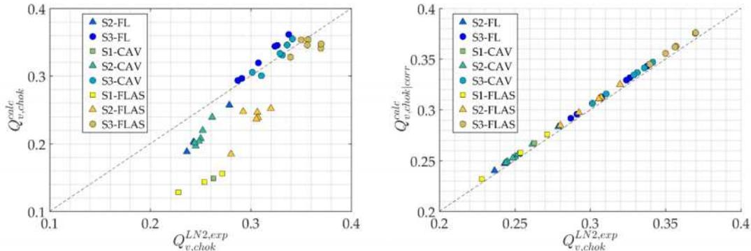
**Figure 4.** Comparison of the cryogenic experimental  $Q_v$  at choking with respect to the one computed from the hydraulic similitude: (a)  $P_{min} = P_{sat}(T_{up})$ ; (b)  $P_{min} = P_{sat}(T_{up}) \cdot f(\Delta T_{sub})$ .
