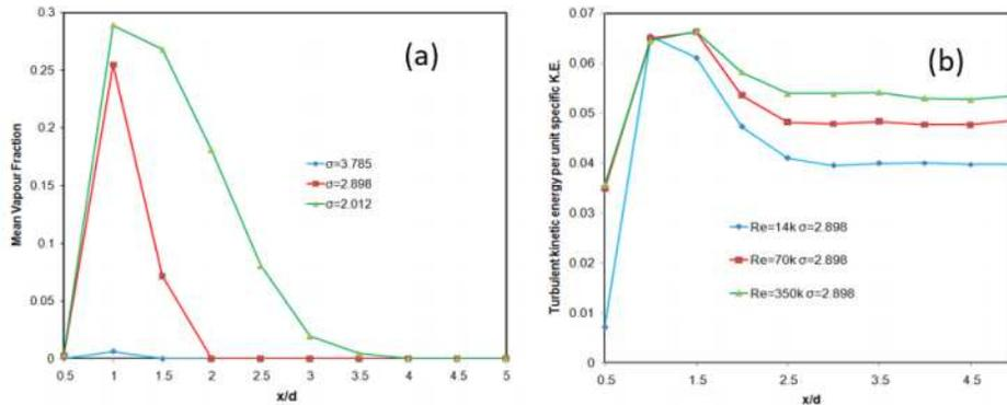
**Figure 4.** (a) Mean vapour fraction vs  $x/d$  for different cavitation number at  $Re_D=14k$ . (b) Turbulent kinetic energy (TKE) per unit specific kinetic energy vs  $x/d$  for different  $Re_D$  at  $\sigma=2.898$ .
