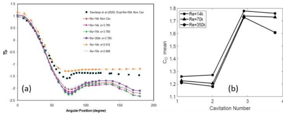
**Figure 3.** (a) Variation of mean pressure coefficient on the cylinder surface  $\overline{C_p}$  for different  $Re_D$  and cavitation number. (b) Mean drag coefficient vs cavitation number for different  $Re_D$ .
