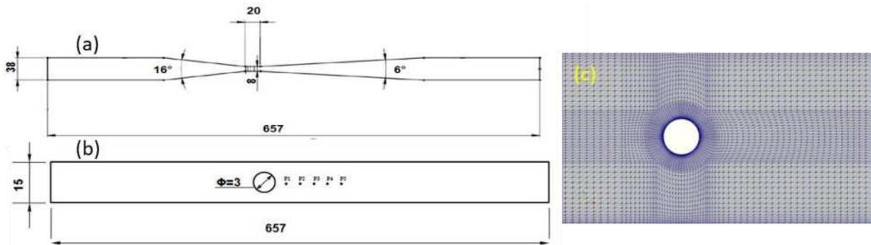
**Figure 1.** Schematic of the computational domain (a) is the front view and (b) is the top view of the domain. P1 to P5 shows the axial location of probes at a fixed distance of  $0.5d$ . (c) Zoomed view of High-resolution O-grid near the cylinder. All dimensions are in mm.
