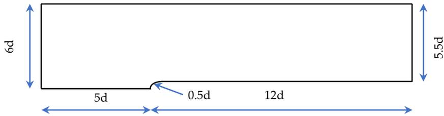
Figure 1. Computational domain for hemispherical forebody projectile
