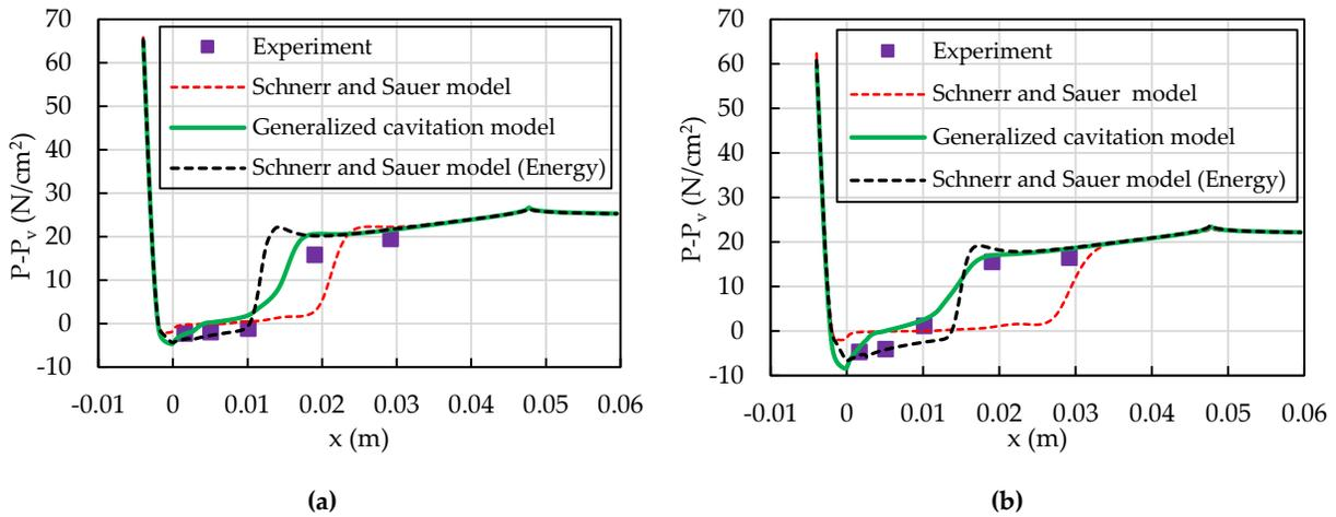
**Figure 4.** Comparison of pressure depression with experimental data of [9] on hydrofoil surface for (a) 290C (b) 296B
