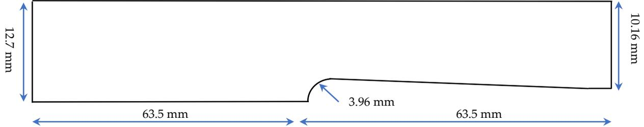
**Figure 3.** Computational domain for hydrofoil
