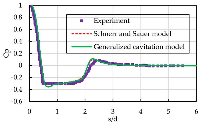
Figure 2. Comparison of pressure variation with experimental data of [8] at  $\sigma = 0.3$
