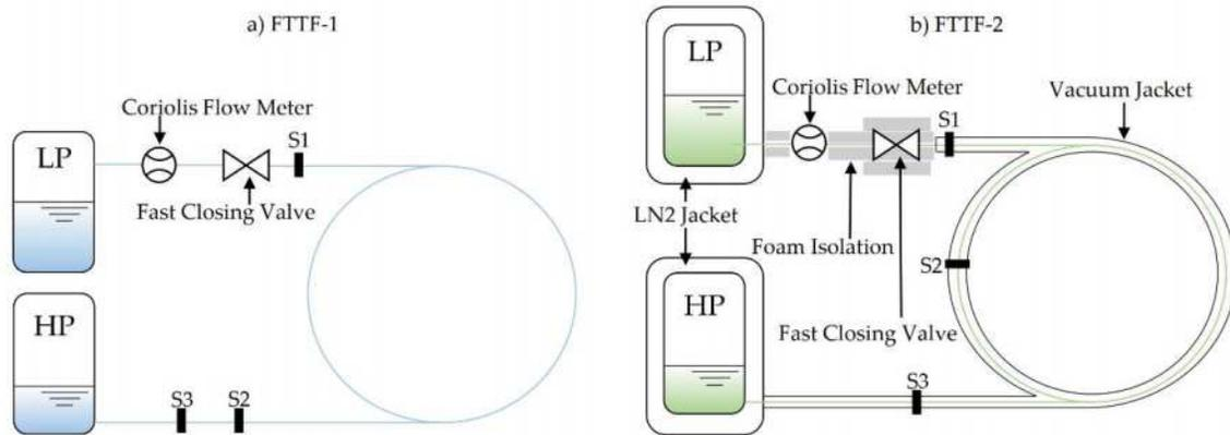
**Figure 1:** Schematic of the FTTF - 1/2. Left: H2O configuration without isolation. Right: LN2 configuration with isolation.
