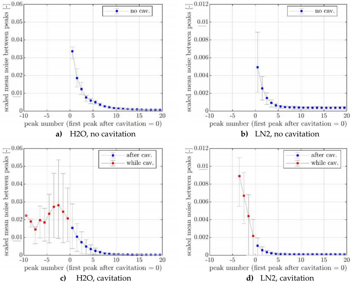
**Figure 3:** Averaged amount of normed noise between peaks for **a)** H2O, no cavitation, **b)** LN2, no cavitation, **c)** H2O cavitation, **d)** LN2 cavitation. The traces are cut after 20 peaks without cavitation.
