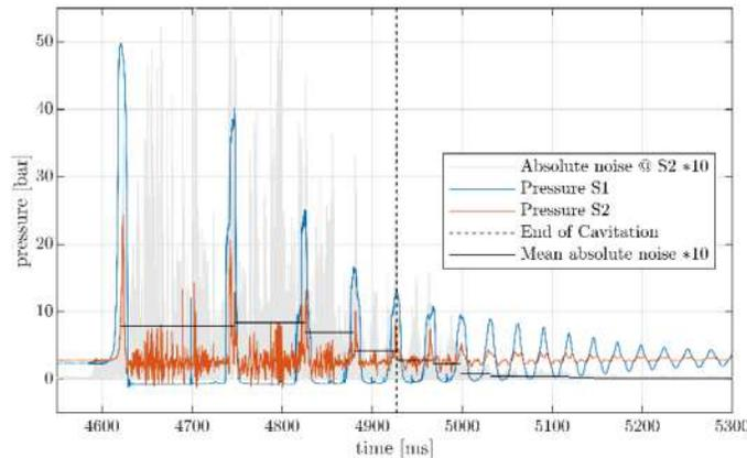
**Figure 2:** Pressure trace at Sensor S1/S2 for H2O. The plot is split into two areas with the dashed line, before and after cavitation. The mean amount of noise is shown between each peak.
