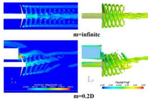
Figure 7. Vortex structure at phase  $\varphi=0^\circ$  of the backward operation condition ( $Q=5000$  1/s<sup>2</sup>).
