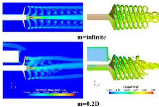
Figure 6. Vortex structure at phase  $\varphi=0^\circ$  of the forward operation condition ( $Q=5000$  1/s<sup>2</sup>).
