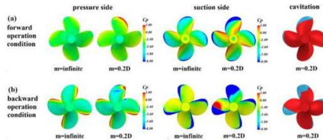
Figure 4. Pressure contour on propeller at phase  $\varphi=0^\circ$
