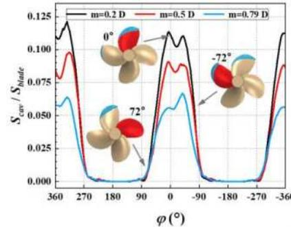
Figure 5. Development of the cavity on the key blade
