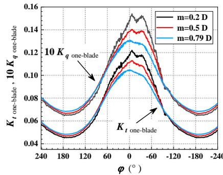
Figure 3. Variation of thrust and torque coefficient for the key blade
