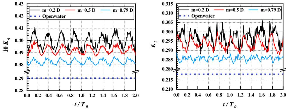
Figure 2. Time history of the thrust and torque coefficient ( $J=0.45$ ) with different distance between ice and propeller
