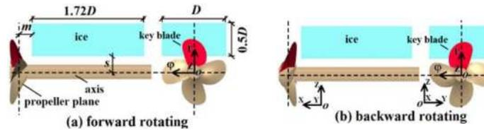
Figure 1. Position of the propeller and the ice
