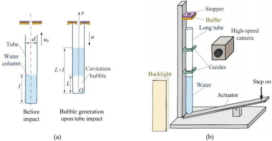
**Figure 1.** Experimental setup. (a) Cavitation bubble generation process by the tube-arrest principle and major parameters (dimensions not to scale); (b) Schematic of the modified tube-arrest apparatus.
