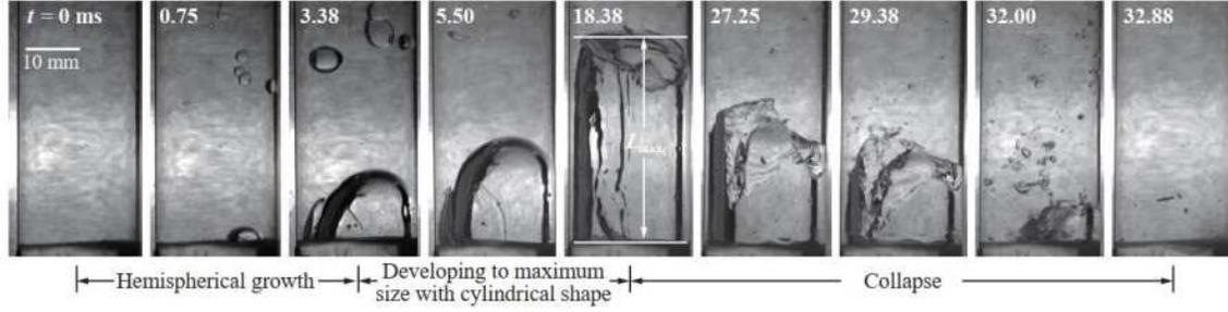
**Figure 2.** High speed images of a typical large cylindrical cavitation bubble formed at the bottom of the tube.  $t = 0$  ms indicates the moment of tube impacting upon the stopper.
