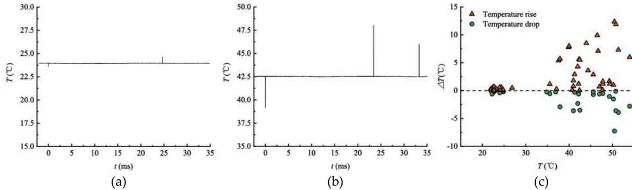
**Figure 3.** Measured results of the thermocouple. (a) 24.0 °C. (b) 42.5 °C. (c) Temperature drop and temperature rise of the first collapse under different temperature conditions.
