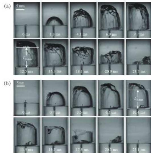
**Figure 2.** High speed images of cylindrical cavitation bubbles at different temperatures. (a)  $T = 24.0$  °C. (b)  $T = 42.5$  °C.
