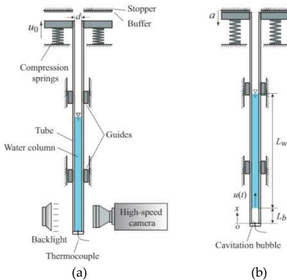
**Figure 1.** Schematic diagram of the tube-arrest principle. (a) Tube moves upward with velocity  $u_0$  before impact with stopper, (b) Cavitation bubble occurs immediately upon tube impact with acceleration
