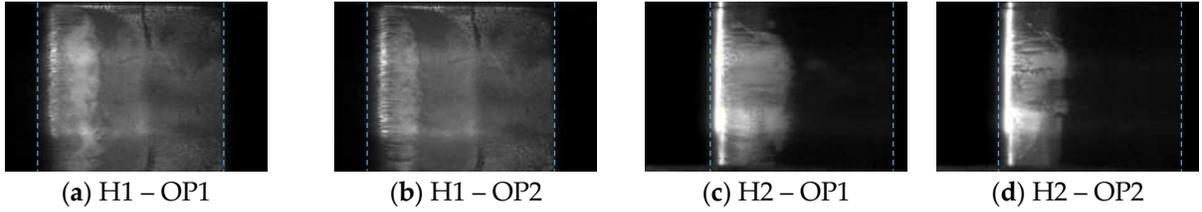
**Figure 1.** Cavitation at hydrofoil H1 and H2 (OP1 – Strong cavitation; OP2 – Medium cavitation).
