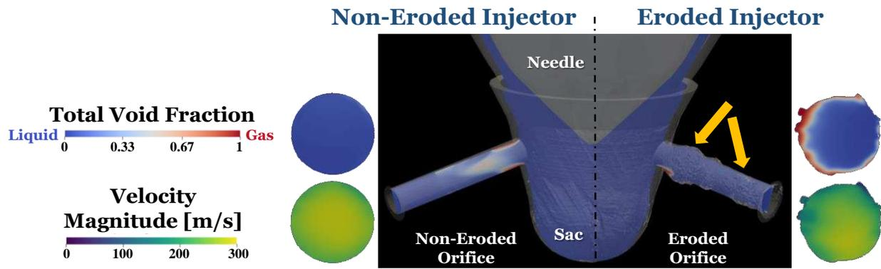
Figure 2. High-resolution x-ray scans of an eroded multi-hole injector conducted at Argonne’s Advanced Photon Source revealed erosion damage in the injector orifices, as indicated by the yellow arrows. Comparison of the predicted injection conditions from the non-eroded orifice (left) and eroded orifice (right) highlight the impact of erosion on cavitation formation, injection velocity, and ultimately fuel delivery rate.
