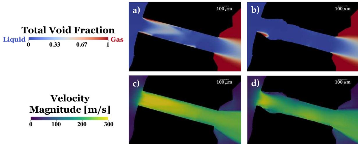
**Figure 3.** A comparison of the predicted flow development for (a-b) total void fraction and (c-d) velocity magnitude distributions for the non-eroded and eroded injector geometries respectively. The visualizations are shown along the central slice at the time instant of maximum needle lift.
