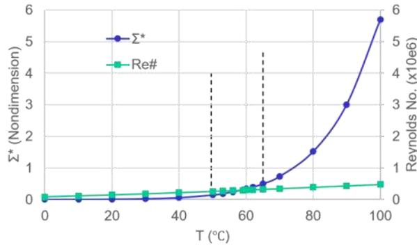
Figure 4. Thermodynamic parameter and Reynolds number changing with temperature
