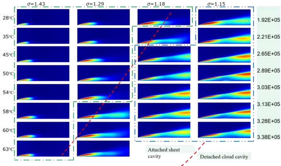
Figure 2. Cavitation topology for cases at different cavitation number and temperatures
