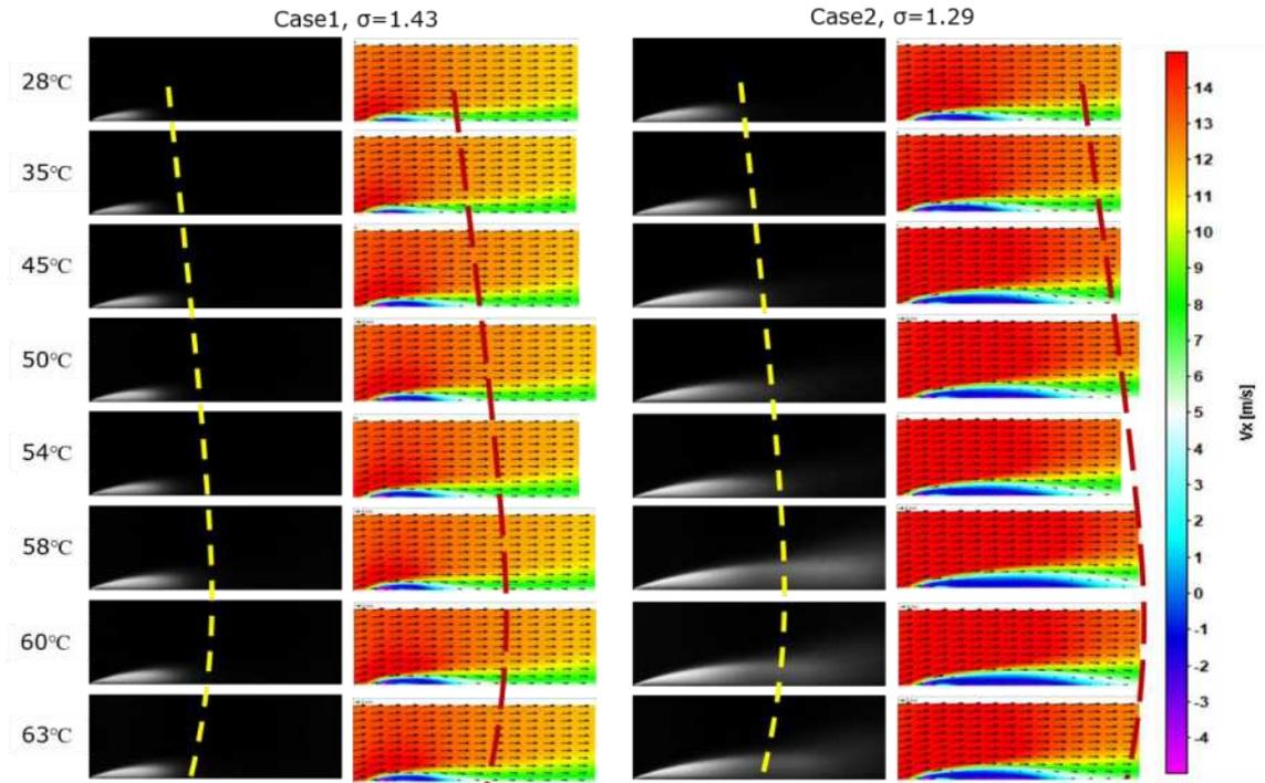
Figure 3. The trend of cavitation length changing as temperature increasing
