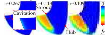
Figure 3.  $f_v$  on blade suction surface in meridional view at different  $\sigma$  conditions
