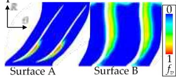
**Figure 7.** The average vapor volume fraction in critical cavitation condition
