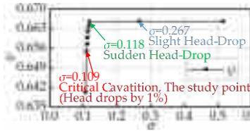
Figure 2. Cavitation performance by CFD
