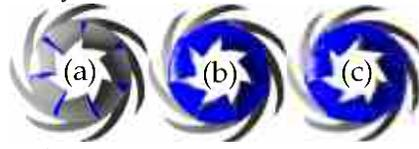
Figure 4.  $f_v > 0.01$  in axial view from impeller inlet direction (a)  $\sigma = 0.267$ , (b)  $\sigma = 0.118$ , (c)  $\sigma = 0.109$
