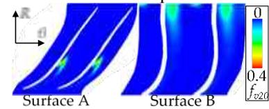
**Figure 9.** Vapor volume fraction amplitude distribution of 20 Hz
