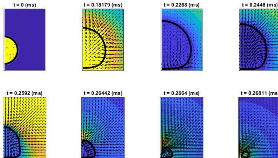
**Figure 2.** Simulation of a nonspherical air bubble with  $h_0 = 1.5R_0$  showing the shape evolution, velocity vectors, and pressure contours in the near-wall region during growth, collapse, and jet impact. A rigid boundary is located along the bottom edge. Blue indicates low pressure and yellow indicates high pressure.
