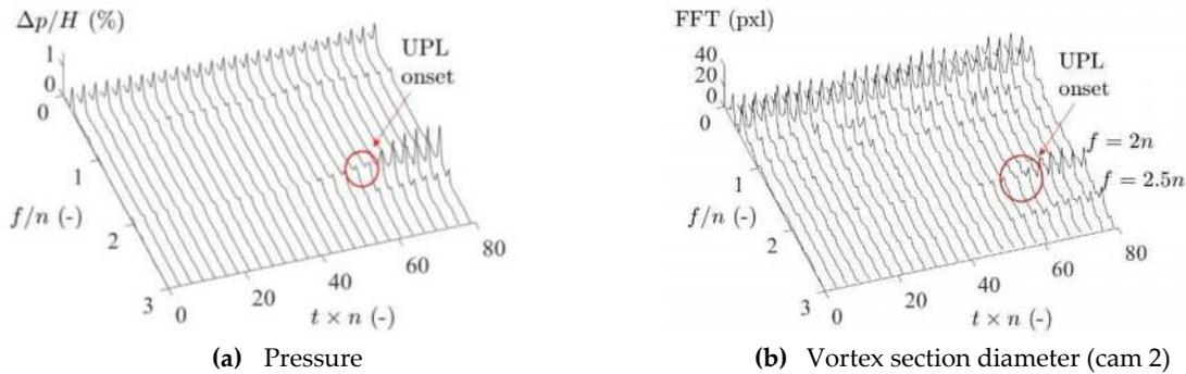
Figure 6. Waterfall diagram of FFT of pressure signal ( $p_1$ ) and vortex section diameter ( $z = 0.12 \times L_{DT}$ ) over time
