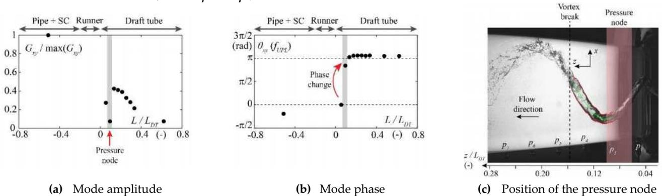
Figure 4. Amplitude and phase mode in the draft tube excited at  $f_{UPL}$
