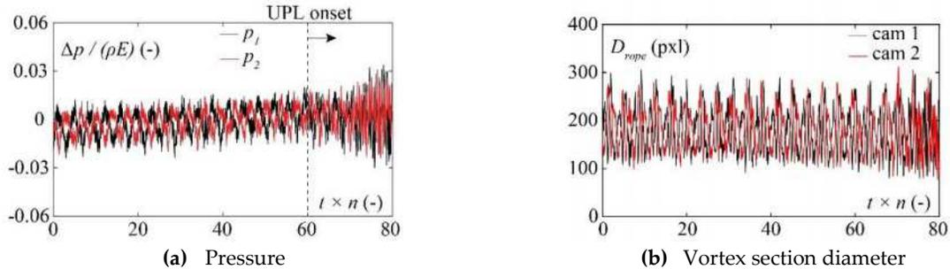
Figure 5. Time history of pressure ( $p_1$  and  $p_2$ ) and vortex section diameter ( $z = 0.12 \times L_{DT}$ )
