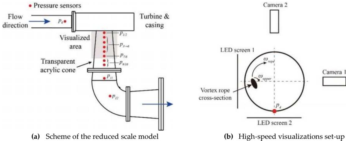
Figure 1. Francis turbine model and experimental set-up.
