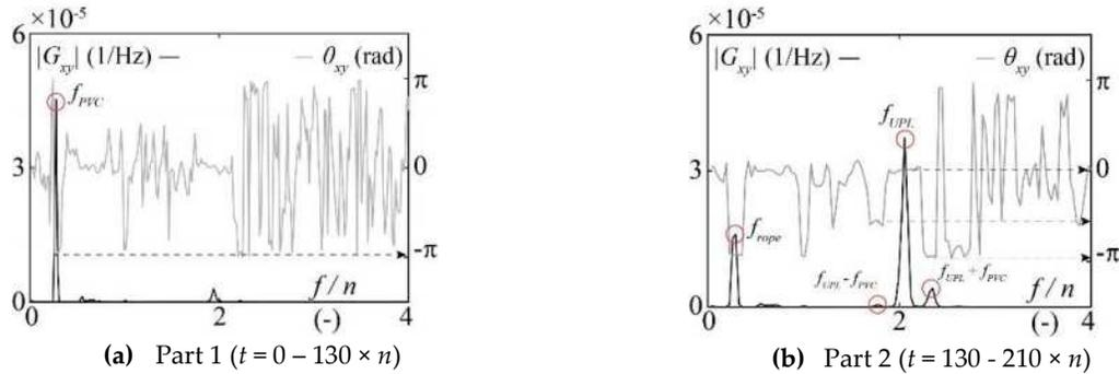
Figure 3. Cross-spectral density function amplitude and phase of two pressure sensors located in the same cross-section (sensors  $p_1$  and  $p_2$ )
