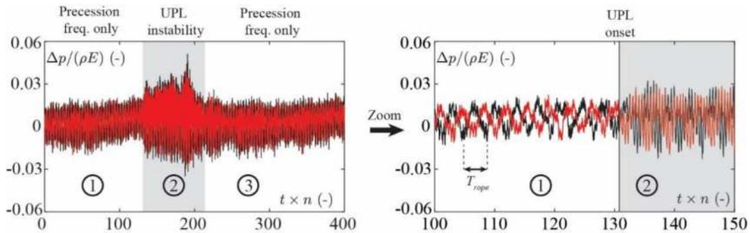
Figure 2. Pressure fluctuations signals in the draft tube cone during UPL instability onset.
